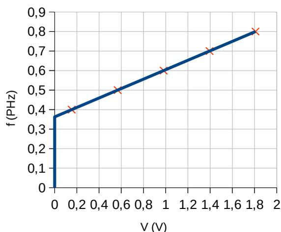
$$m = \frac{(8,000 - 4,000) \cdot 10^{14} [\text{Hz}]}{(1,809 - 0,154 [\text{V}])} = 2,417 \cdot 10^{14} \text{ Hz/V}$$
