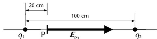
$$\vec{E}_{P_1} = 9,00 \cdot 10^9 [\text{N} \cdot \text{m}^2 \cdot \text{C}^{-2}] \frac{2,00 \cdot 10^{-6} [\text{C}]}{(0,200 [\text{m}])^2} \vec{i} = 4,50 \cdot 10^5 \vec{i} \text{ N/C}$$
